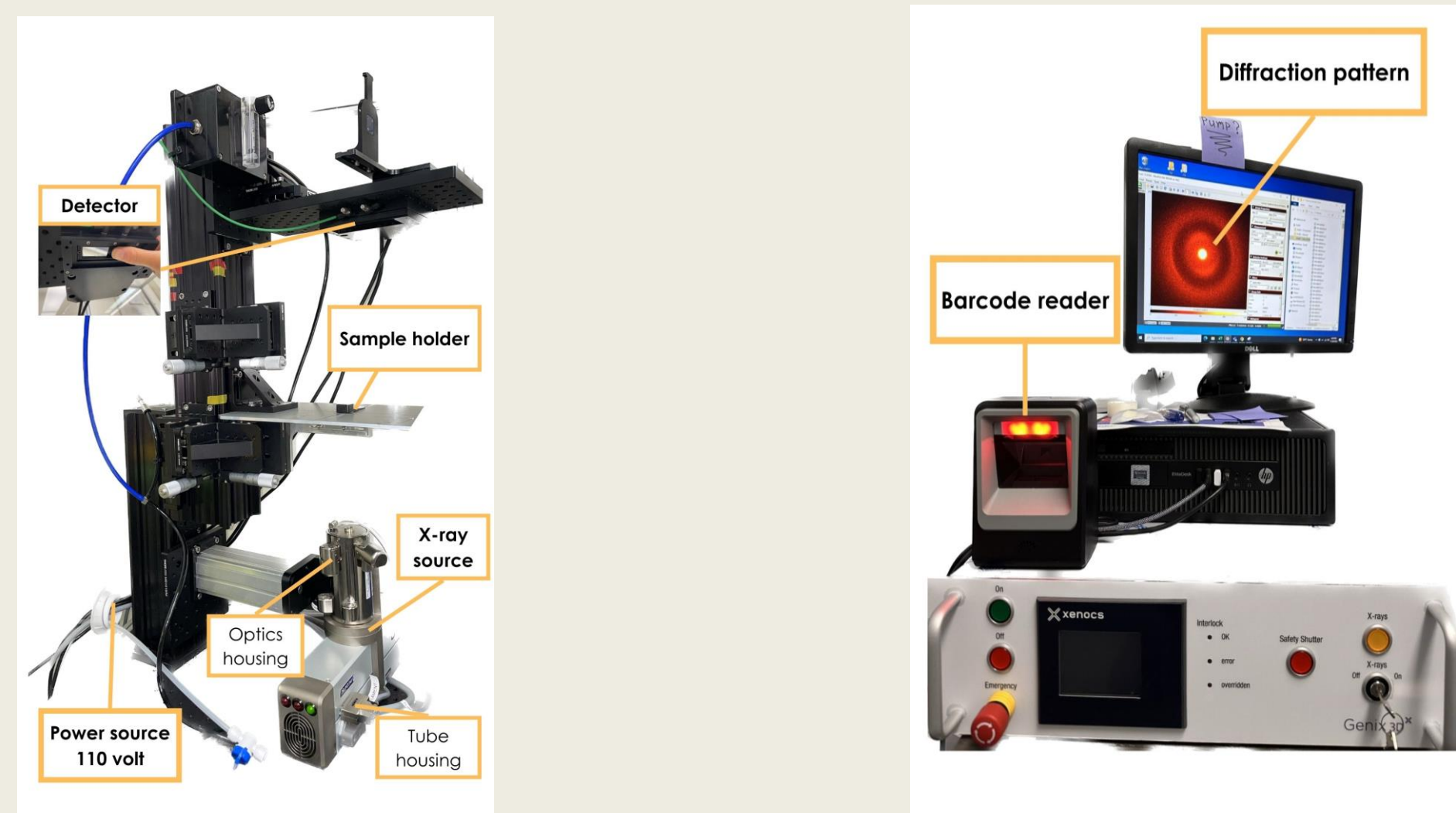
Fig 2: XRD instrument used at EosDx
